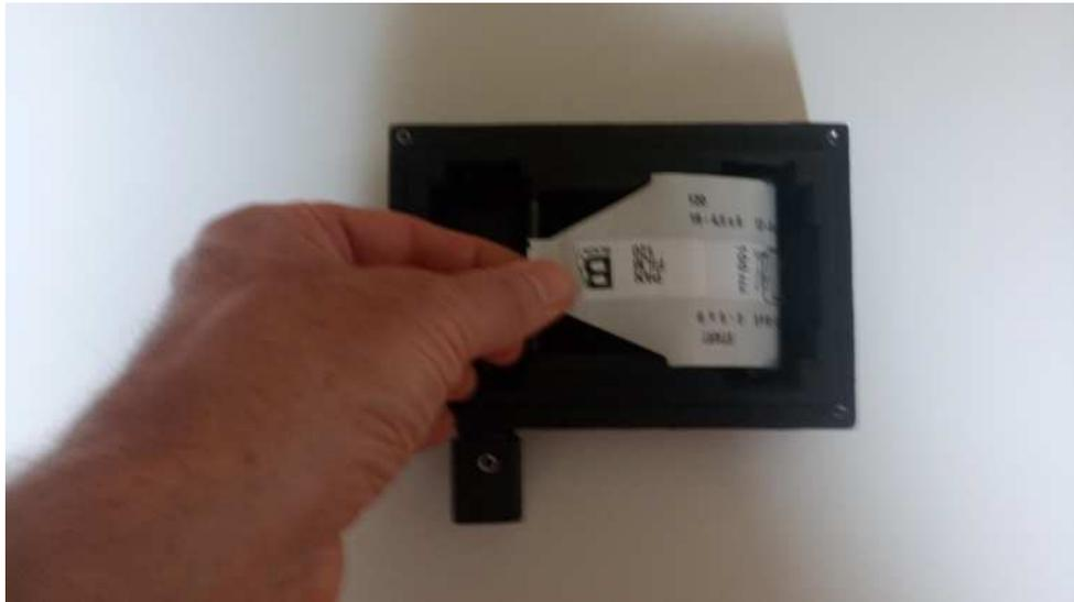
Insert the back paper into the vertical slot of the empty coil and then rotating the knob 3 to wind the back paper around the empty coil. Executing two or three knob rounds to verify that back paper is winded correctly.
